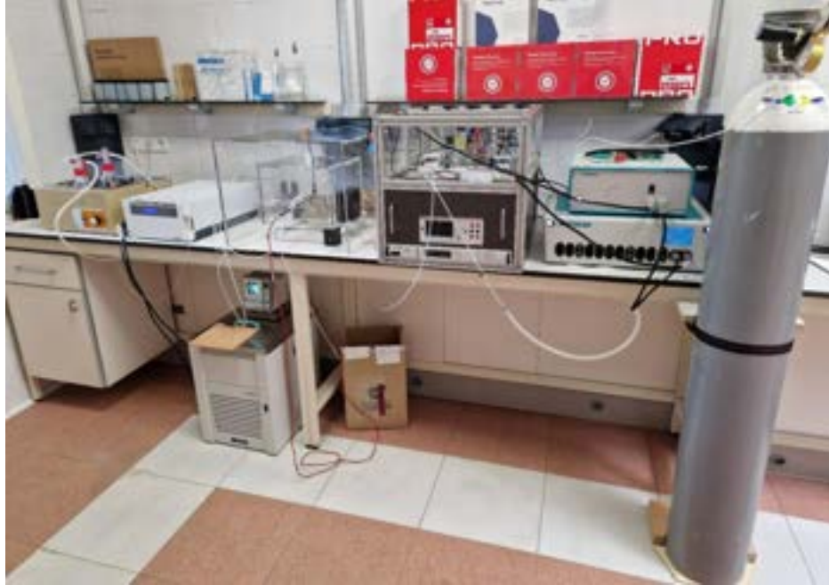
Figure 2. The test bench designed and built to study DMFC and methanol electrolyzers.
