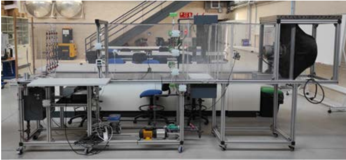
Figure 3: Subsonic wind tunnel facility in which the experimental tests are carried out.
