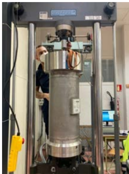
Figure 5: High pressure hydrogen chamber for material testing.
