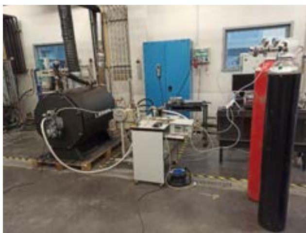
Figure 8: Combustion chamber CO 2 lung (combustion tests of the ternary mixture CH 4 /CO 2 /H 2 ).
