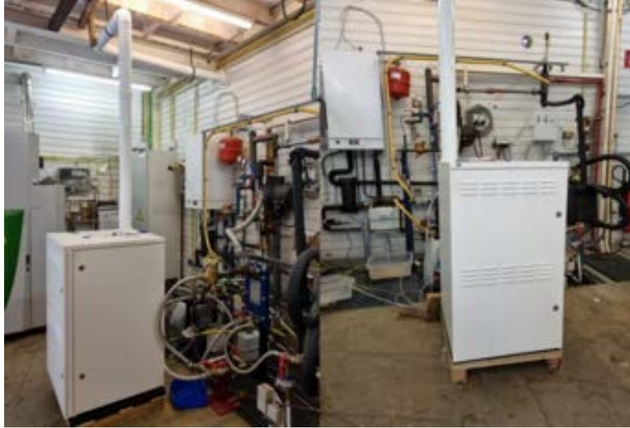
Figure 1. Tested mCHP SOFC in ULiege laboratory facilities
