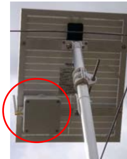
Figure. 7. Omnidirectional antenna installed in the peripheral towers.
