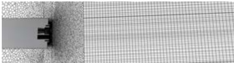
Figure 5. Example of mesh in axial cut plane of whole kiln mesh.
