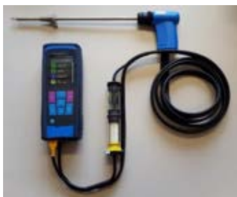
Figure 3. 'Multizyzer STx' combustion analyser portable meter
