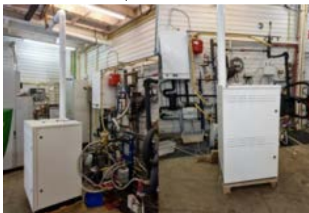
Figure 2. Tested mCHP SOFC in the laboratory facilities of the University of Liege
