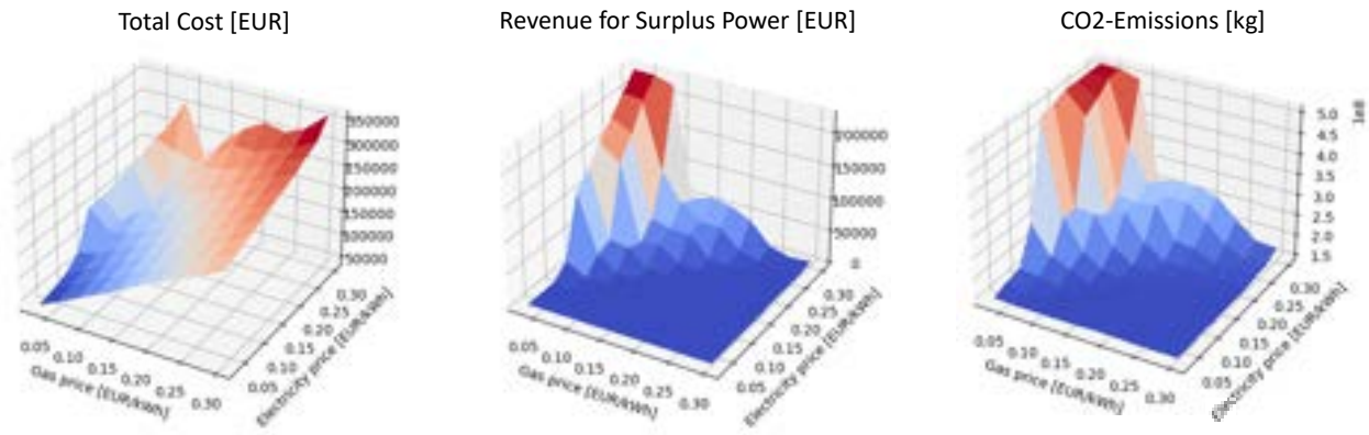
Figure 4: Optimization results for December 2021: Total cost, revenue for surplus power and local CO 2 -emissions for a parameter-grid of varying gas and electricity costs
