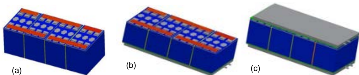
Figure.5. Battery module thermal management: a) module without any cooling plate, b) module with bottom cooling plate, c) module with top and bottom cooling plates
