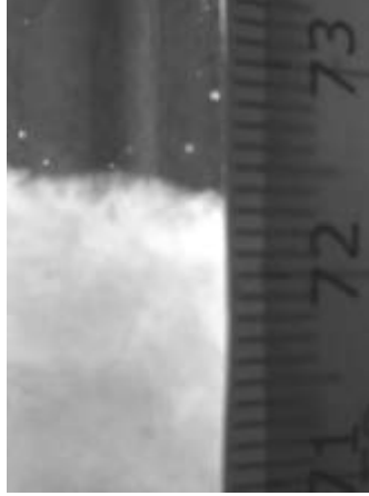
Figure 5. Picture of the phase change front during melting, taken with the camera installed next to the tube in tube heat exchanger ( x = 72.4 cm).
