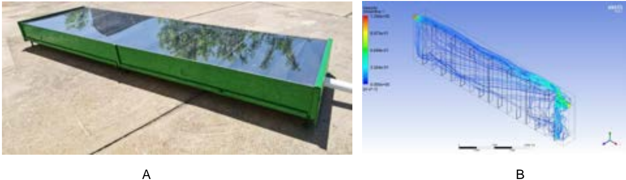
Figure. 10. Solar air collector validation: A – Experimental validation prototype; B – ANSYS Fluent thermofluidic analysis and optimization model.
