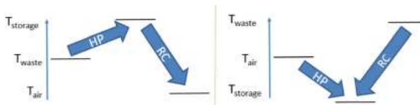
Figure. 1. Hot storage configuration versus cold storage configuration [4].
